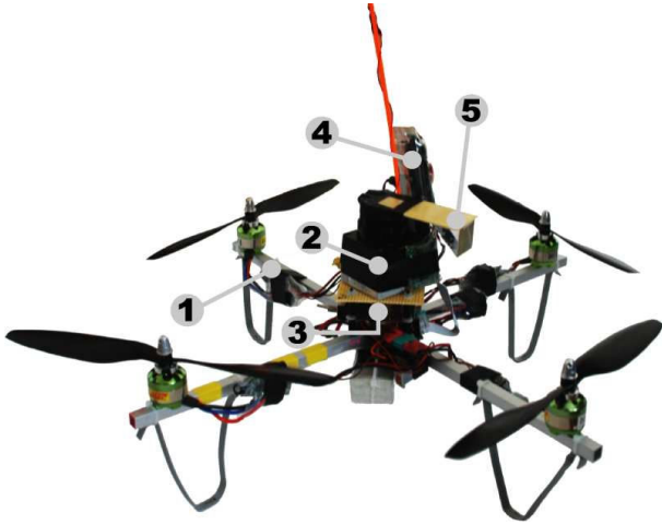
Fig. 2. The quadrotor platform used to evaluate the navigation system includes a Mikrokopter (1), Hokuyo laser range finder (2), an XSens IMU (3), a Gumstix computer (4), and a laser mirror (5).
